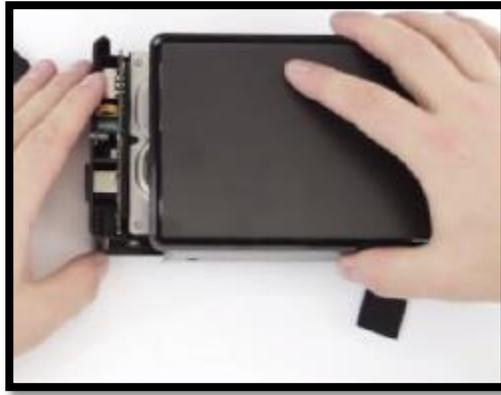
The hard drive is held together by Phillips screws on both sides. You will need to use your Phillips screw driver to remove the screws that are found on both sides of the hard drive.
